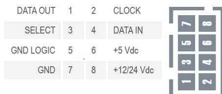
The connector is pin-to-pin compatible with the one on the AL66 FG coin selectors
